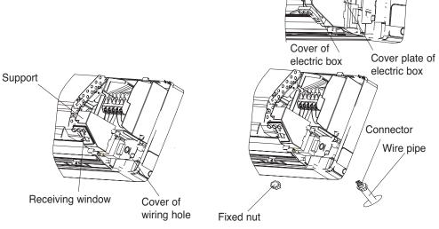
4. Wire pipe should be tightened by the fixed nut and the electric box should be fixed as shown in the above right figure and the below figure.
